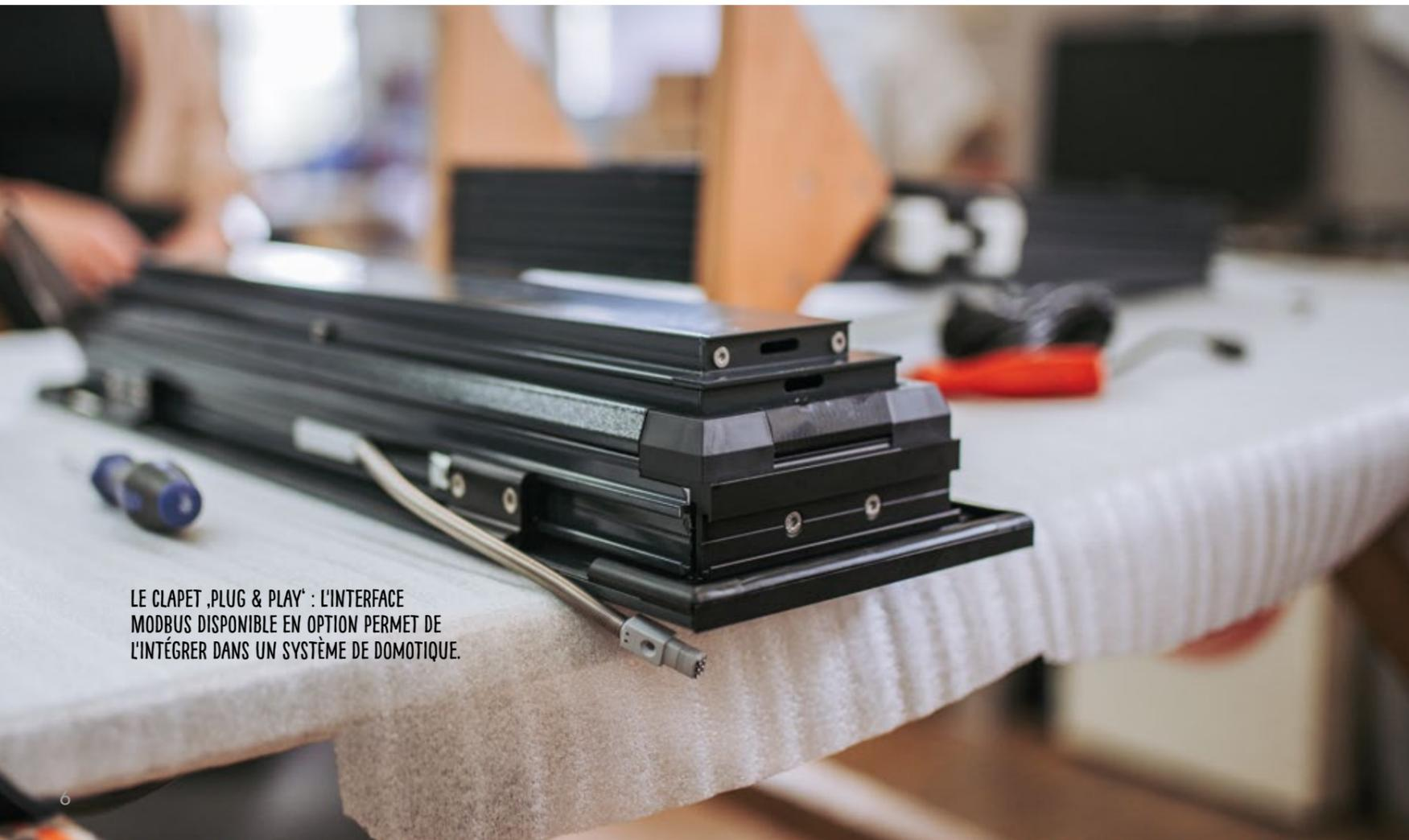
**LE CLAPET 'PLUG & PLAY' : L'INTERFACE MODBUS DISPONIBLE EN OPTION PERMET DE L'INTÉGRER DANS UN SYSTÈME DE DOMOTIQUE.**
